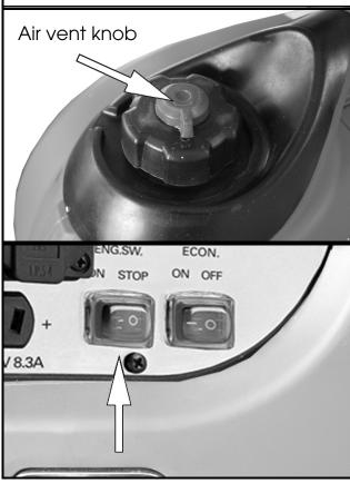
4. Set the engine switch to the "0" (OFF) position.
