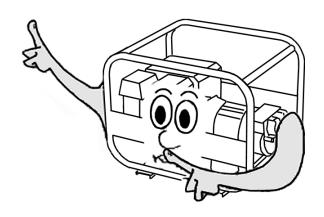
5. **Never** start the engine if there is spilled fuel. Any spillage must be wiped clean and the generator allowed to dry before attempting to start the engine.
